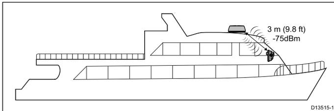
In the example above the maximum distance with acceptable Wi-Fi performance was 3 metres (9.8 feet), due to the metal roof that the signal has to pass through.
