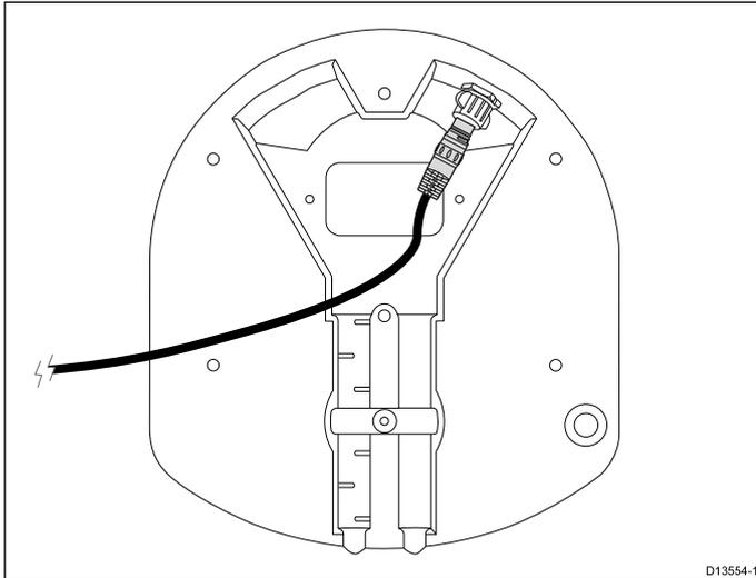
Route the power cable to the side of the unit to allow for the pole mount.
