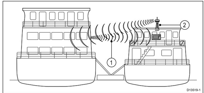
1. In this example the Wi-Fi signal is bounced off a nearby vessel and back through the windows on the bridge, this provides an easier path than passing through the metal roof.
