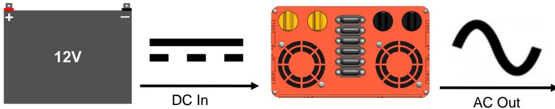
**Figure 10.1** Simple diagram on how the inverter works
