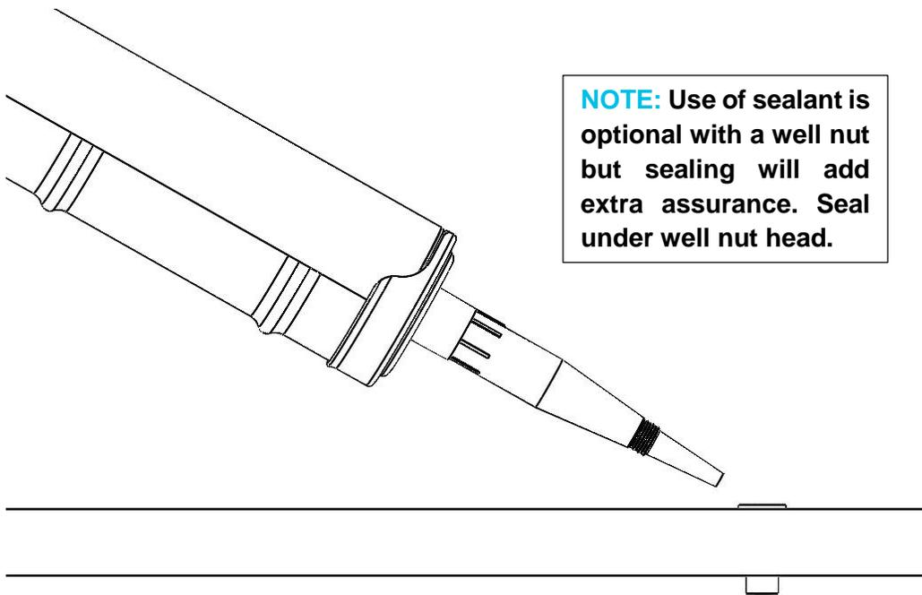
**NOTE:** Use of sealant is optional with a well nut but sealing will add extra assurance. Seal under well nut head.
