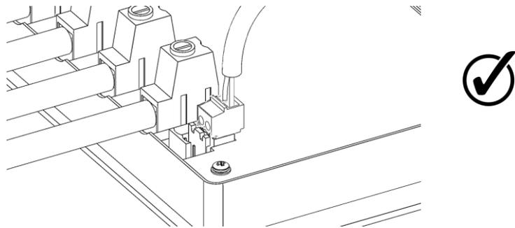
**4. Insert battery remote sensor block terminal and connect wires
