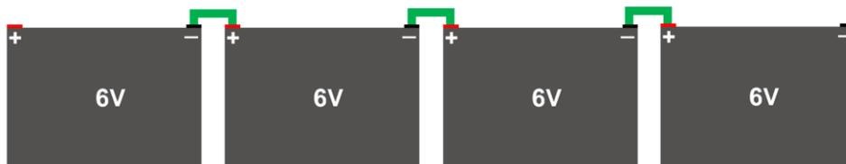
**Figure 9.5** Four 6V batteries connected in series
