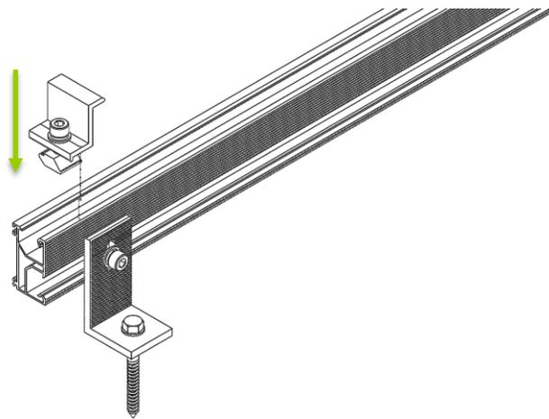
**⚠ WARNING:** End clamps must be installed a minimum of 1" (30 mm) from the rail edges.
