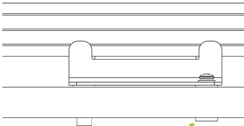
**NOTE:** Screw has compressed and expanded the well nut, binding into the roof material.
