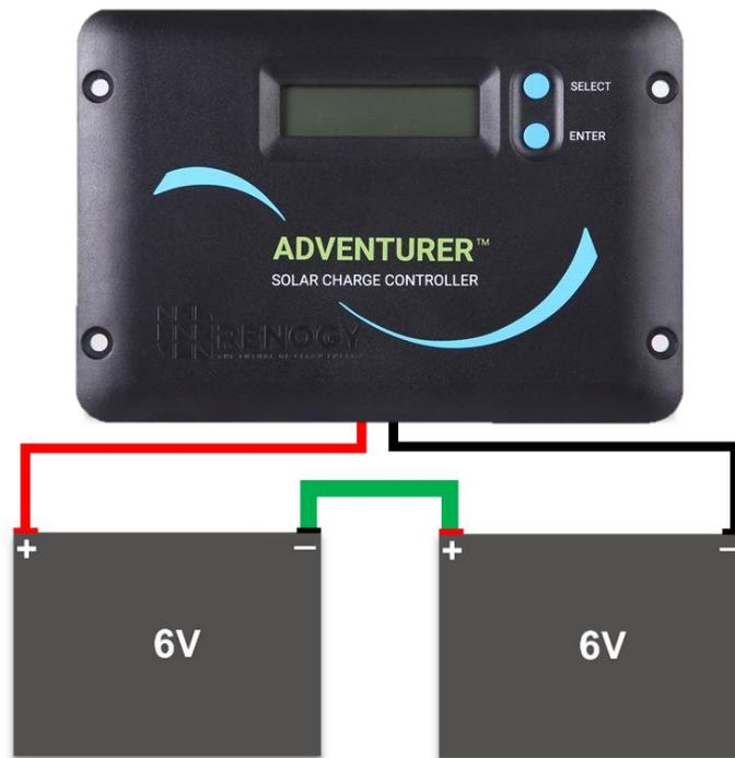
**Figure 9.1** Two 6V batteries connected in series
