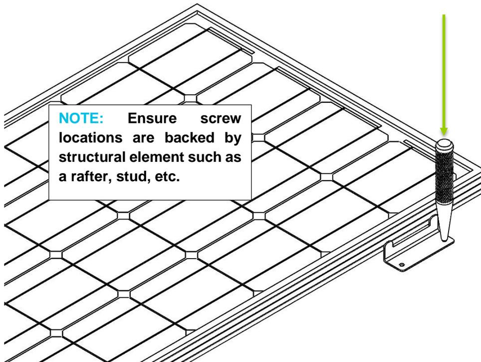
**NOTE:** Ensure screw locations are backed by structural element such as a rafter, stud, etc.
