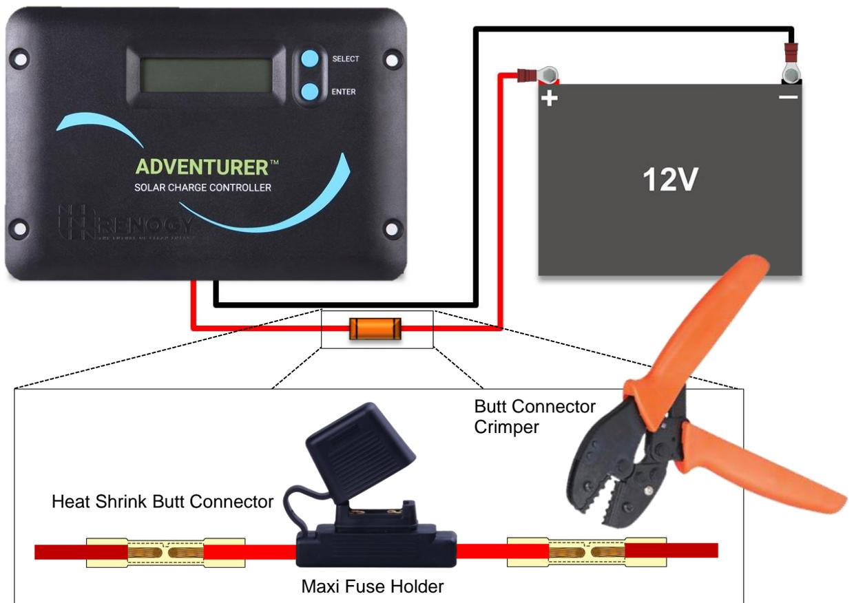
The butt connectors recommended for this application are the type with heat shrink insulation. This will keep will give extra protection for the internal connection.
