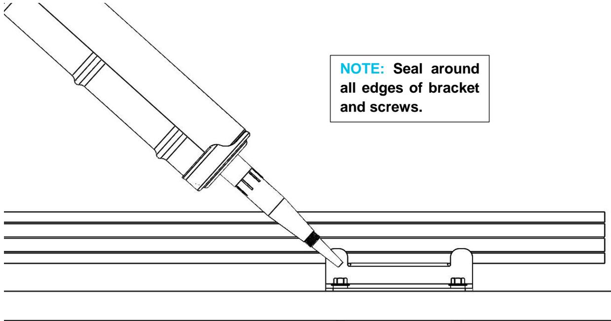
**NOTE:** Seal around all edges of bracket and screws.
