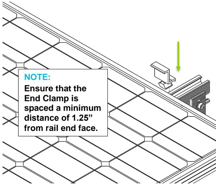
**⚠ WARNING:** End clamps must be installed a minimum of 1" (30 mm) from the rail edges.
