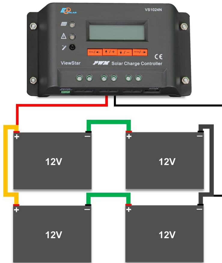
**Figure 9.6** Four 12V batteries connected in series – parallel
