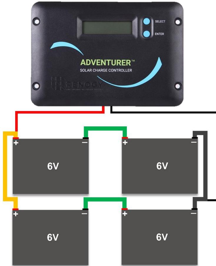
**Figure 9.3** Four 6V batteries connected in series – parallel
