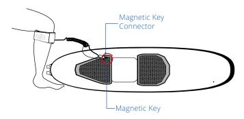
The magnetic key is a security mechanism, the jet will not activate if this key is not properly placed.
