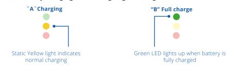
5. The LEDs in the battery will progressively light up as the battery is being charged.
