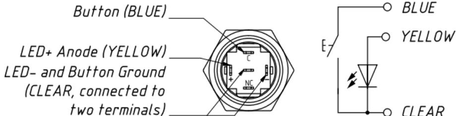
*Figure 2. Button terminals and electrical scheme*
