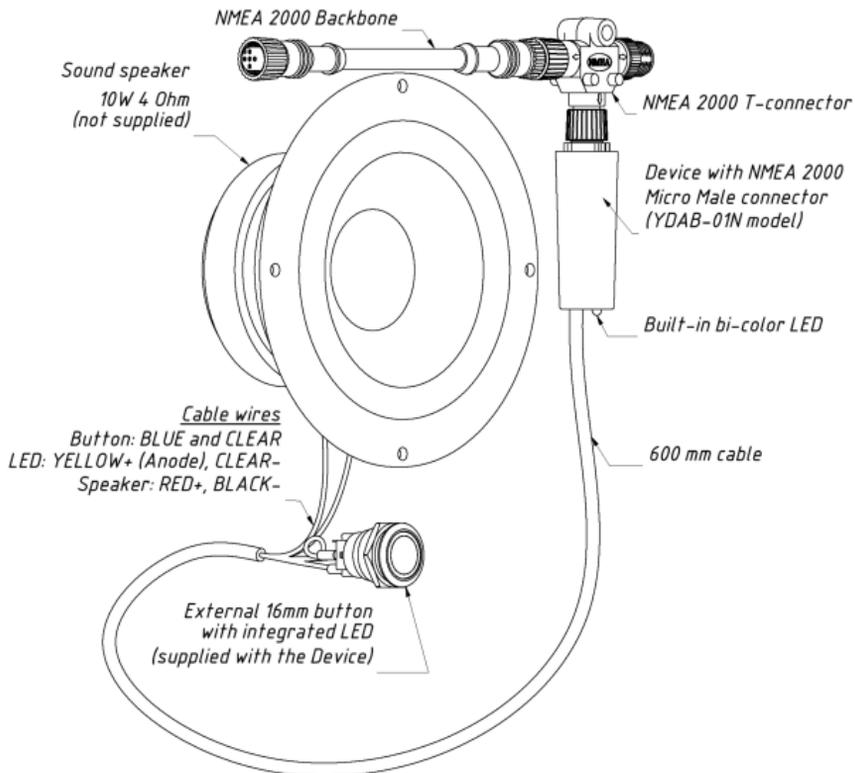
Figure 1. Device connection
