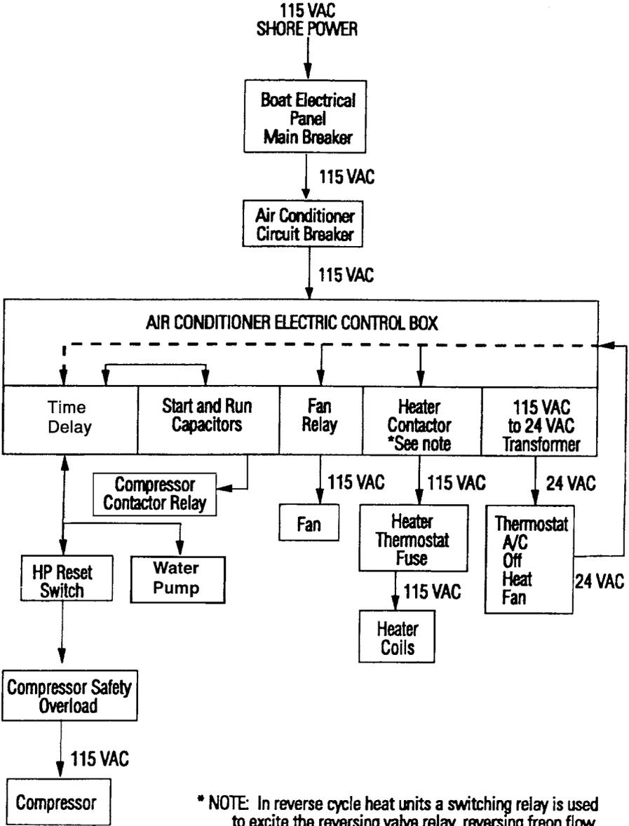
\* NOTE: In reverse cycle heat units a switching relay is used to excite the reversing valve relay, reversing freon flow.
