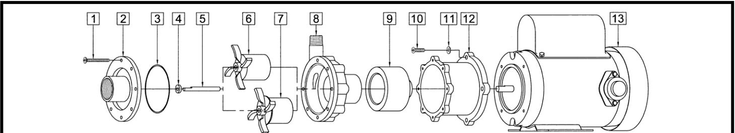
When attaching the Drive Magnet to motor shaft, position the face of the Drive Magnet 3/32 inch below the face of the Motor Bracket.
