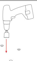
Using a hole saw, cut a hole for the electronics cable.
