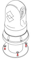
Insert the four nylon washers into the base bolt holes. Apply marine adhesive sealant around the nylon washers.
