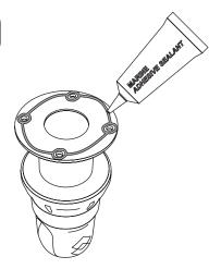
Apply marine adhesive sealant around the bottom of the mount. Be sure to go around the bolt holes.
