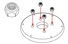
Insert the four nuts into the top plate of the PM5-FMH-8.
