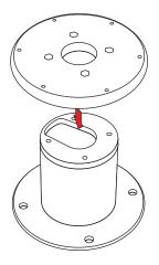
Place the top mounting plate onto the PM5-FMH-8. Be sure that the four mounting holes are lined up.
