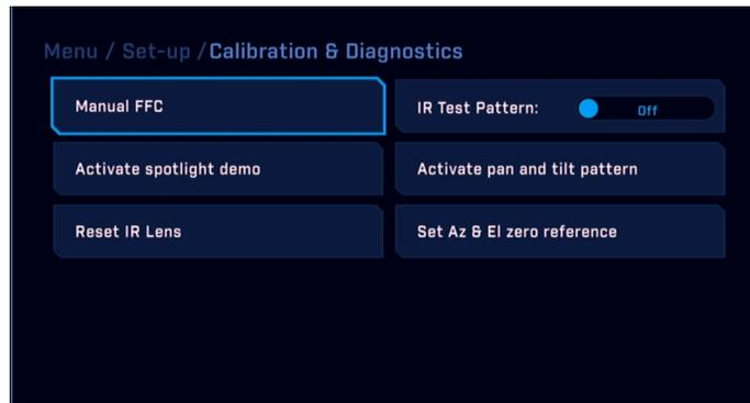
**Manual FFC** This function applies to the IR camera only. When selected, the camera drives the camera to a preset position and performs the FFC calibration (< 5 s). The camera then returns to its Home position.
