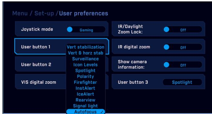
**Joystick mode:** Gaming/Pilot) In managing the elevation (tilt) of the camera, the joystick can be used in one of two modes.
