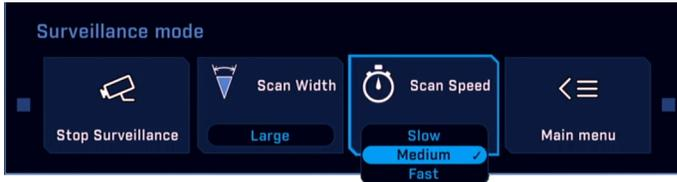
**Scan Width:** In surveillance mode, the Scan Width determines the range of horizontal azimuth (pan) covered by each scan. The choices are:
