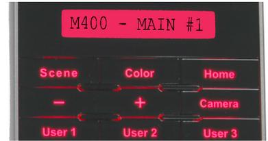
**Short Press**—A short press of the Scene button cycles through the four preset AGC settings, which change the image gain and level settings. The icon for each scene preset is shown on the video monitor display.
