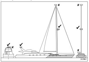
The scanner must also be mounted where it is:
