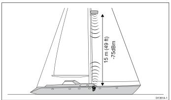
In the example above the maximum distance with acceptable Wi-Fi performance was 15 metres (49 feet), due to the heavy fiberglass coach roof that the signal has to pass through.
