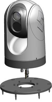
Top-down installation using mounting plate
