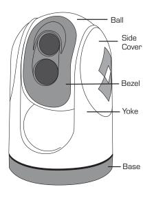
designed for the harsh outdoor environment and have a coating for durability and anti-reflection, but may require cleaning occasionally. FLIR Systems Inc. suggests that you clean the lens when image quality degradation is noticed or excessive contaminant build-up is seen on the lens.
