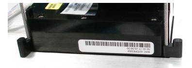
If you intend to mount the JCU to a panel of 0.79 cm (0.31 in) thickness or less, remove the clamps from the mounting screws, turn them around and thread them back onto each of the four screws. In this configuration, the clamp foot faces the
