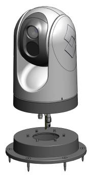
Top-down installation using riser
