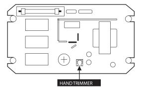
Figure 32: Hand Trimmer Location on AVR.
