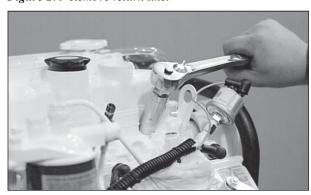
Figure 18: Unscrew injector.
