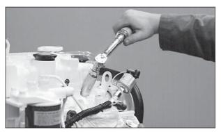
Figure 20: Reinstall injector. Torque to proper tightness.
