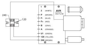
Figure 28: Voltage Selector Terminal, 240 Volt Output b. Connect U2 to V1 on the output terminal board (Figure 29).
