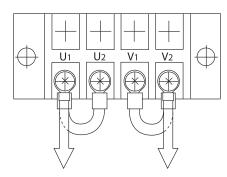
Figure 27: Output Terminal Board, 120 Volt Output
