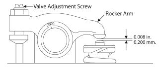
Figure 10: Valve Adjustment
