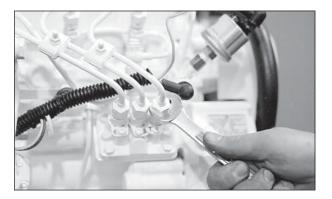
Figure 13: Remove delivery line flare nuts.
