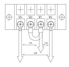
Figure 31: Output Terminal Board, 120/240 Volt Output
