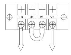
Figure 29: Output Terminal Board, 240 Volt Output
