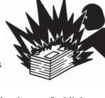
Never check battery charge by contacting the posts with a metal object. Use a volt-meter or hydrometer.
