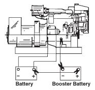
**Figure 22:**Battery connections.
