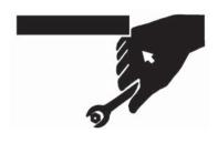
Use power tools only to loosen threaded parts and fasteners. For loosening and tightening hardware, always use the correct sized tools. Do not use US measurement tools on metric fasteners, or vice versa. Use only service parts that meet Northern Lights specifications.
