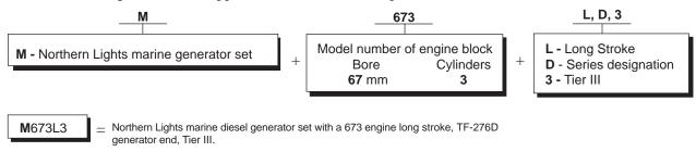
M673LD3 = Northern Lights marine diesel generator set with a 673 engine long stroke, TF-276D generator end, Tier III, 5 kW.
