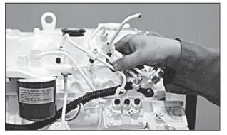
Figure 14: Remove delivery lines.
