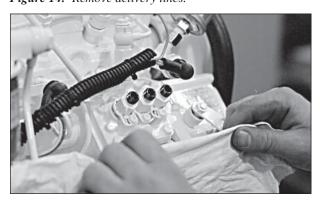
Figure 15: Cover lines, inlets and injection pump outlets.
