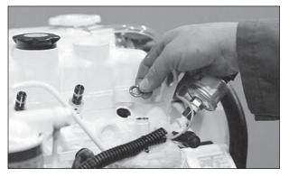
Figure 19: Remove and replace copper sealing washer.
