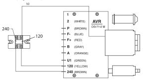
Figure 26: Control Terminal Board, 120 Volt Output
