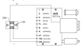
Figure 30: Control Terminal Board, 120/240 Volt Output
