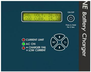
Figure 10 – Front Panel Display
