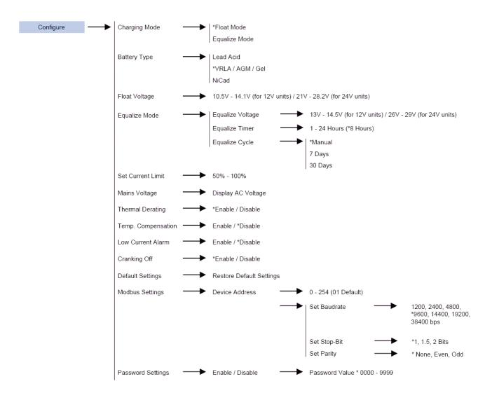
Figure 11 - MSM Configuration Mode
