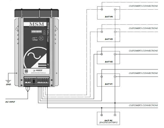
Figure 6 - Typical MSM System Configuration Shown with Optional 5 Battery Charger Divider
