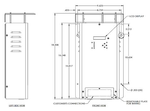
Figure 2 – MSM Mounting Dimensions for Medium Case #203
