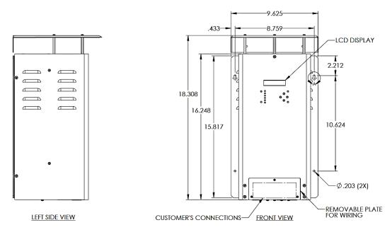
Figure 3 - MSM Mounting Dimensions for Large Case #205
