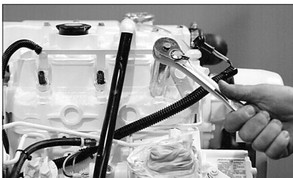
**Figure 15:** Unscrew injector.
