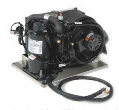
This unit is available in right, left or top air discharge configurations, and is now available as a cool reverse cycle heat unit., We use 4" ducting and recommend a minimum of 2, 4" round supply grills with this installation.
