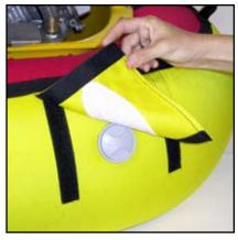
1. Lift Velco  ${}^{\scriptscriptstyle\rm TM}$  flap on the side of the tube cover.
