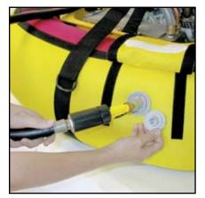
4. Located at the end of the black heat hose is a male QRS fitting which fits snugly into the clear tube. With the compressor running, insert the male QRS fitting into the clear tube and begin filling.
