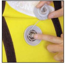
7. Deflation is very quick and easy. Remove the valve cover by turning counter clockwise and simply depress the quick-deflate button in the center of the valve. You may also lock the valve open by depressing the quick-deflate button and turning it clockwise. Replace valve cap, turn clockwise to secure. Press fabric cover back into place. Turn engine off until you are ready to launch the unit.
