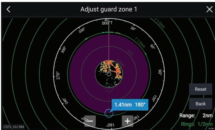
Adjust the guard zone's size by dragging the inner and outer perimeter end points (circles) to the desired locations.
