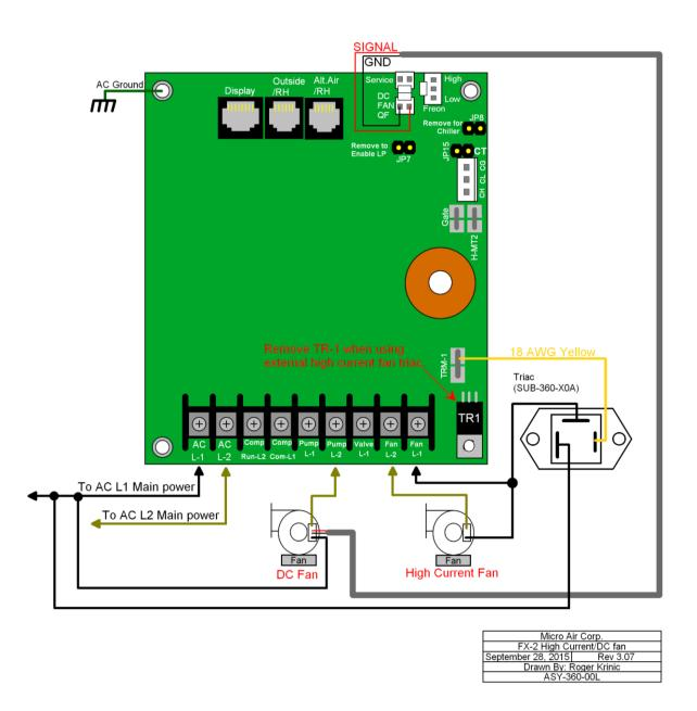
*Note:* Up to two DC fans can be connected to the DC fan output.
