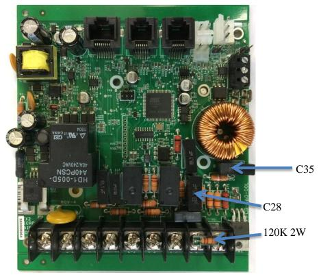
Remove C35 and C28 for contactor or pump relay connected to fan output. Install a 120K 2W resistor on fan L1, L2.
