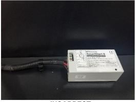
INCORRECT (horizontal surface, water could intrude into case)
