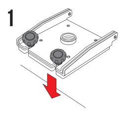
Place the hinge adapter onto the surface you are going to mount to.
