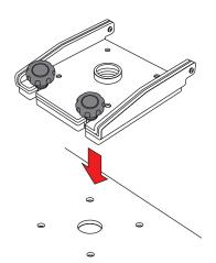
Place the hinge adapter onto the mounting surface. Make sure to lineup all the bolt holes.
