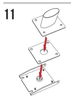
Place the foam gasket (included in your Seaview mount) and the Seaview mount onto the top hinge adapter plate.
