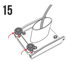
Fold the knobs back over and tighten to secure the two plates of the hinge adapter.
