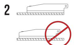
Be sure that the hinge adapter is placed near the edge of the surface to allow for adaquate room to hinge back.
