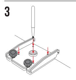
Mark the four bolt holes to drill, along with the center cable hole.
