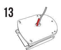
Route the electronics cable through the hinge adapter and through the Seaview mount.
