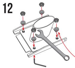
Apply some marine adhesive sealant to the four nylon shoulder washers. Then put them on the four bolts securing the Seaview mount to the hinge adapter.
