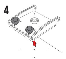
Remove the hinge adapter from the mounting surface.
