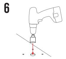
Using a 2" hole saw, cut a hole for the cables.
