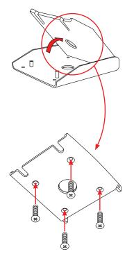
Insert the four 5/16-18 X 1" bolts through the underside of the top hinge adapter plate.
