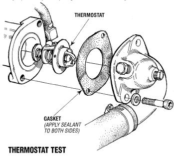
If you suspect a faulty thermostat, place it in a pan of water and bring to a boil. A working thermostat should open about 1/2"
