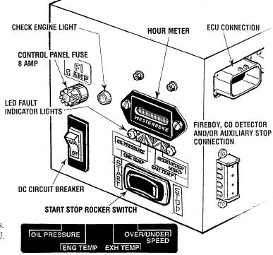
The Ext. Alarm indicates a faulty fire suppression circuit. By-pass the circuit to determine the fault (the fire suppression circuit must be closed when the circuit is running).
