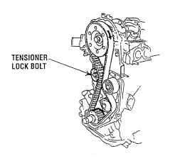
CAUTION: Water or oil on the timing belt severely reduces the service life of the belt. keep the timing belt sproket and tensioner free of oil and grease. These parts should never be cleaned. Replace if seriously contaminated with dirt or oil. If oil is evident on these parts, check the front case, oil pump seals, and camshaft oil seals for a possible leak.
