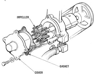
**CAUTION:** If any of the vanes have broken off the impeller, they must be found to prevent blockage in the cooling circuit. They often can be found in the heat exchanger.
