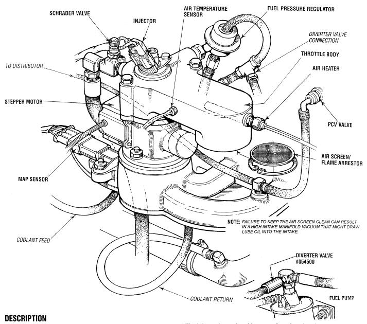
The above illustration shows the throttle body assembly that attaches to the intake manifold.
