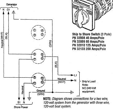
If the installer connects shore power to the vessel's AC circuit, this must be done by means of the Shore Power Transfer Switch. Set the transfer switch shown in the diagrams to the OFF position. This switch prevents simultaneous connection of shore power to generator output.
