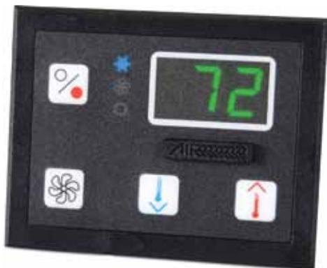
The Passport I/O Environmental Control Unit is a microprocessor based controller, designed for the precise control and monitoring of direct expansion and chilled water boat air conditioning systems from Marine Air. The control is dual voltage, operating at both 115 and 230 Volts, 50/60 Hz. The display is available in both black and white. In chilled water air handlers, the control is referred to as AH-Passport I/O.
