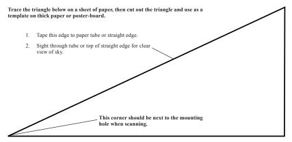
This edge must be kept horizontal at the mounting location
