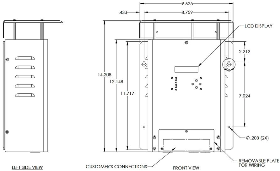
**Figure 1 - MSM Mounting Dimensions for Small Case #201**
