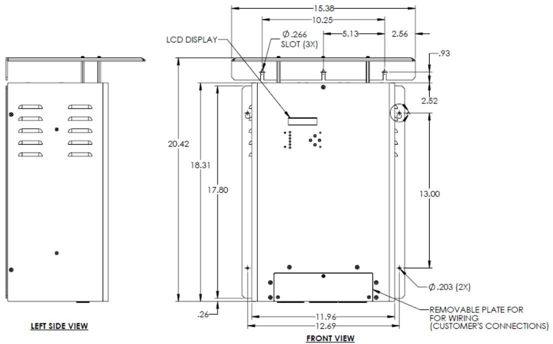
**Figure 4 - MSM Mounting Dimensions for Large Case #207**
