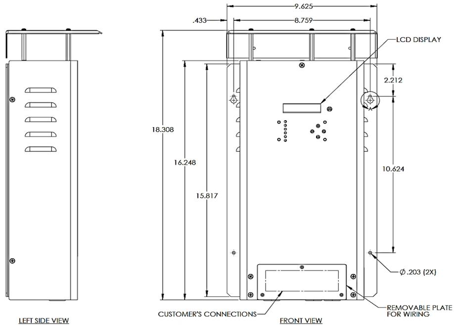
**Figure 2 – MSM Mounting Dimensions for Medium Case #203**
