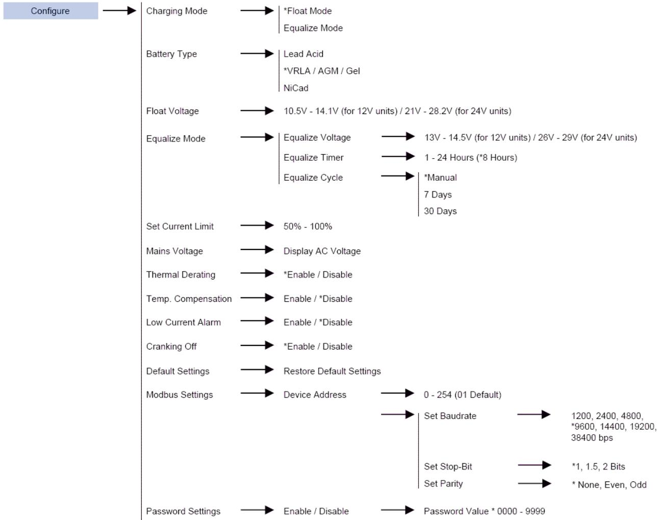
**Figure 11 - MSM Configuration Mode**
