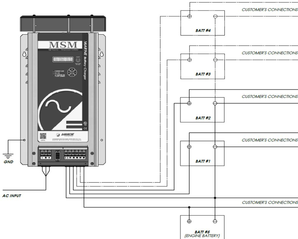
**Figure 6 - Typical MSM System Configuration**
