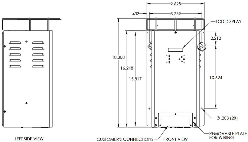
**Figure 3 - MSM Mounting Dimensions for Large Case #205**
