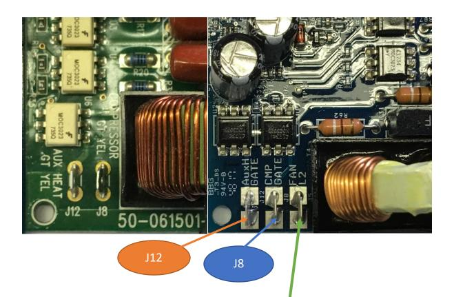
This connection must only be used for fan L2. It improves the fan electrical noise filtration which can be a problem in some systems. Do not connect valve, compressor or pump L2 here or the board may be damaged.
