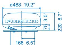
24" Radome Radar Sensor DRS4D-NXT 7.3kg 16.1 lb
