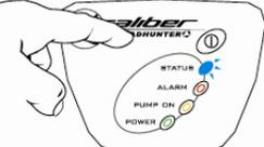
After a performance setting has been selected, push and hold the hidden mode switch for 8 seconds until the **blue** LED flashes to enter the routine for setting the cut in pressure.
