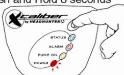
To accept the cut in pressure, and performance settings and exit from the pump set-up routine; push and hold the on/off switch for 8 seconds until the power LED returns to the **red** "standby" mode.
