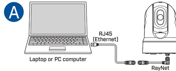
Note: Power connections are not shown. Each device requires its own power connection.
