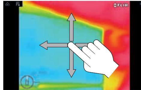
On a touchscreen multifunction display you can pan, tilt, and zoom the thermal camera image using the touchscreen:
