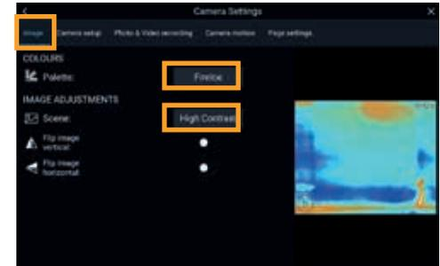
A range of color palettes and scene presets are available to help you distinguish objects on-screen in different conditions. With the thermal camera application displayed:
