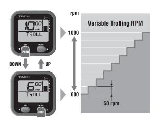
By just pressing a button on the optional Command Link® tachometer, the operator can adjust the engine's trolling speed from 600 ~ 1000 rpm, in 50-rpm increments. This helps provide precise and consistent trolling speeds in a wide array of conditions.
