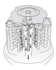
Yamaha's exclusive "In-Bank" exhaust system exits downward through the center of the engine between the "V" of the cylinders, rather than on the exterior side. This increases combustion efficiency for more power and torque, and also provides for a more compact shape.
