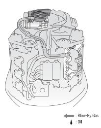
Yamaha V MAX SHO outboards feature a Blow-by Gas Re-Burning System. This separates any unburned combustion gases and re-routes them to the air intake system where they are burned again, helping maximize fuel efficiency and earn a CARB 3-star emissions rating.
