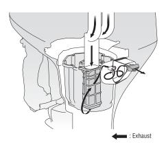
Engine exhaust is routed through a maze before exiting above the waterline through the idle exhaust relief outlet, for unbelievably smooth and quiet operation. A mufflerless design creates a more direct exhaust flow and a pleasing sound of power at idle.
