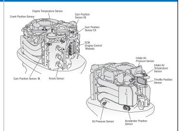
A multitude of advanced sensors constantly provide vital atmospheric and engine conditions to the Engine Control Module (ECM), which instantly makes the precise adjustments for optimum performance, durability, and efficiency.
