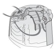
The V MAX SHO features an advanced cowling drain system, to easily and efficiently drain away any water that enters the cowling during normal engine operation. Incoming air is routed through a labyrinth of passages that trap and drain water before it enters the engine's intake, for maximum reliability.
