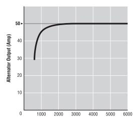
With 46 amps of total alternator power at 1000 rpm and a full 50 amps from 2000  $\sim$  6000 rpm, V MAX SHO outboards offer the kind of charging power needed to help operate today's wide array of on-board electronic devices.
