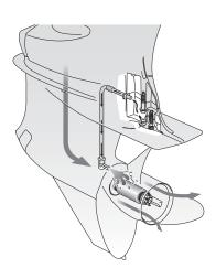
V MAX SHO outboards have an exhaust pressure reduction system, which not only helps keep the propeller hub cooled from hot exhaust gases, it also helps provide power by "forcing" those gases out of the engine during the critical hole shot and acceleration phases.
