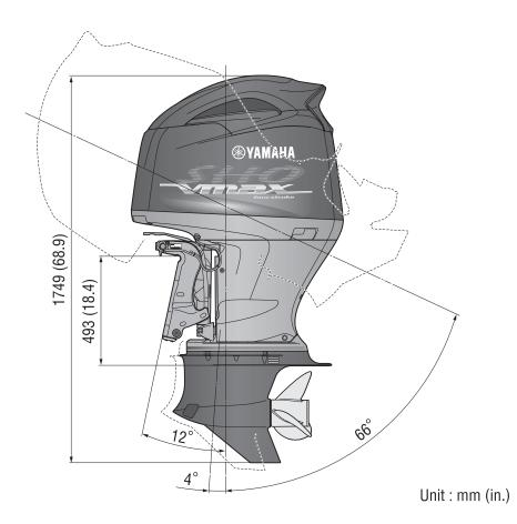
The break-through four stroke technology used in Yamaha's new V MAX SHO help keep exterior dimensions surprisingly compact, and the 35° maximum steering angle to the left or right gives you excellent control.
