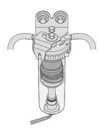
All V MAX SHO outboards utilize a large, on-engine water separating fuel filter with a water sensor. Used in conjunction with Yamaha's 10-Micron Water Separating Fuel Filter, it helps separate water and contaminants from the fuel before they can reach the outboard's other filters and fuel injectors.
