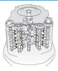
4.2 liters of class-leading displacement teams with individual intake and exhaust camshafts to provide more precise valve timing control with fewer moving parts than conventional rocker arm systems for increased reliability. This superior design also allows for use of 4 valves per cylinder which exchange intake and exhaust gases more efficiently for responsive power and increased fuel economy. Intake valves are 14% larger and exhaust valves are 10% larger than our 3.3L DOHC system.
