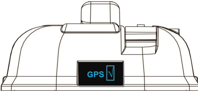
In Self-Test, the display illustrates the test result of each step with “√” indicating a pass and “X” indicating a failure. There are a total of five tests, plus a battery check. If all tests pass, SELF-TEST PASS will be displayed at the end of the Self-Test mode. This will be followed by the GPS coordinates horizontally scrolling through the display, provided the beacon has successfully downloaded an external GPS location. See Appendixes B through E for details about display messages.
