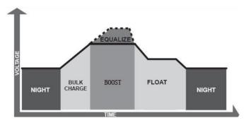
The Voyager charge controller has a 4-stage battery charging algorithm for a rapid, efficient, and safe battery charging. They include: Bulk Charge, Boost Charge, Float Charge, and Equalization.
