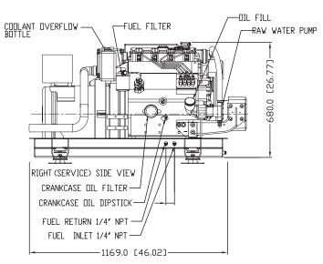
M844LW3 Overall Dimensions L x W x H:  $46.0 \times 22.8 \times 27.5$  inch ( $1169 \times 580 \times 697$  mm) Sound Enclosure Dimensions L x W x H:  $46.0 \times 22.8 \times 28.1$  inch ( $1169 \times 580 \times 714$  mm) Sound Enclosure Weight: 90.0 lbs. (40.9 kg)
