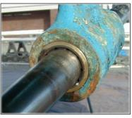
The above photo shows how cleaning the strut face thoroughly will clearly reveal the bearing outer shell for most accurate measuring.
