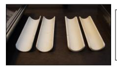
These special non-metallic spacers are provided for 3/4" and 7/8" shafts. They space the 1-1/4" o.d. x 1" i.d. collets away from the shaft to match up the two smallest shafts.
