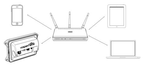
The XB-8000 can also join an existing network. It can do this in either DHCP mode (default) or you can set a static IP address using vmAIS (see configuration section). To prevent the address from automatically changing we recommend that you use a static IP address.
