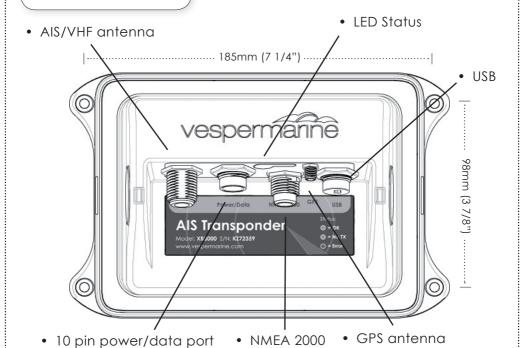
Mount your XB at least 0.6m (2 feet) from any compass. Test your compass to verify that it operates properly when the XB is operating.
