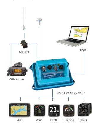
The only AIS transponder with fast 5Hz GPS navigation rate. Use the XB-6000 as your primary GPS source for your NMEA 2000 and NMEA 0183 equipment.
