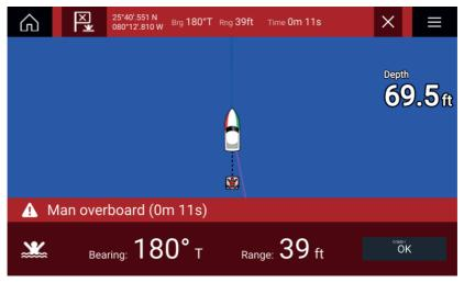
The MOB feature requires your vessel to have a valid position fix from a GNSS receiver. Dead reckoning mode also requires Heading and Speed data.
