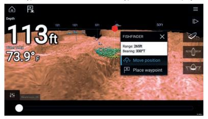
Select Place waypoint to create a waypoint at the marker's location, or Select Move position to adjust the marker's position before creating the waypoint.
