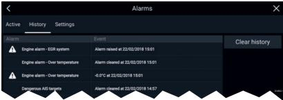
All Dangerous (Red) and Warning (Orange) alarms will appear in the Alarm history list. The history list will include an entry for the alarm being triggered (raised) and also for when the alarm is acknowledged (cleared). The Alarm field contains the name of the alarm and the events field contains details of the alarm condition and its time and date.
