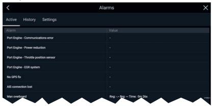
The Active alarms tab lists all alarms that are currently active. Alarms will remain active until the conditions that triggered the alarm are no longer present, e.g.: a Shallow depth alarm will automatically dismiss when the depth becomes deeper.
