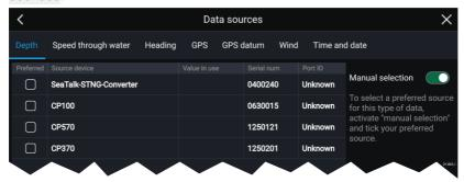
Each tab enables you to view and select your preferred data source. The currently active data source will display its current value in use. Data source selection can be manual or set to automatic:
