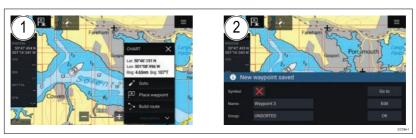
Select and hold on the desired location and select Place waypoint from the context menu.. 2. Select **Edit** to edit the waypoint details, **Goto** to navigate to the Waypoint, or **OK** to return to normal operation.
