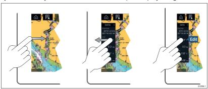
The Sidebar is displayed automatically in the Chart app when a Goto or follow is initiated. It can also be displayed at anytime by sliding your finger from left to right from the left edge of the screen. Swiping right to left will hide the Sidebar.
