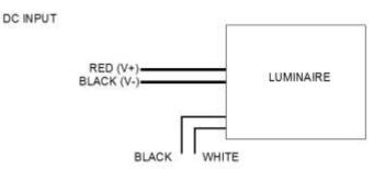
INSTALL A 10K POTENTIOMETER BETWEEN THE BLACK AND WHITE SIGNAL WIRES FOR DIMMING OPERATION. ALTERNATIVELY, SHORT THE SIGNAL WIRES FOR FULL BRIGHTNESS OR LEAVE OPEN FOR FULL DIMMING.
