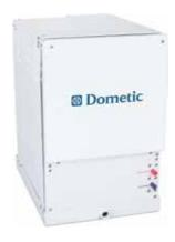
Maximize chiller efficiency and reduce electrical load fluctuations with Dometic's innovative Variable Capacity Chiller (VARC48). At full speed, the VARC48 provides a nominal four tons of cooling or heating. It also has the ability to modulate its speed all the way down to one ton in order to precisely match demand.
