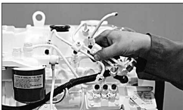
Figure 14: Remove delivery lines.
