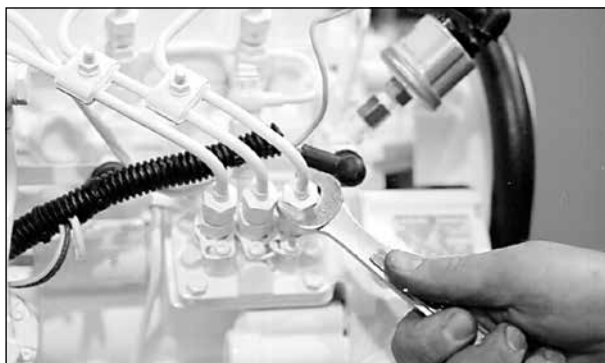
Figure 13: Remove delivery line flare nuts.
