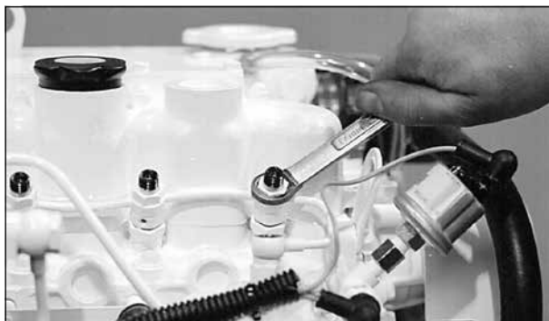
Figure 16: Remove return line nuts.
