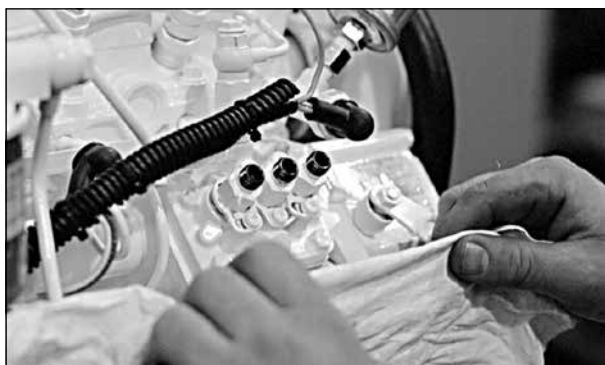
Figure 15: Cover lines, inlets and injection pump outlets.
