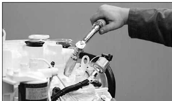
Figure 20: Reinstall injector. Torque to proper tightness.
