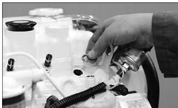
Figure 19: Remove and replace copper sealing washer.
