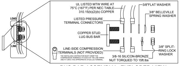
USE ONLY 75°C (167°F) COPPER CONDUCTORS ONLY ON ALL FIELD INSTALLED LINE, LOAD TERMINATIONS INTENDED FOR USE WITH TERMINATED CONDUCTORS.
