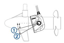
2 Tighten the knob or mounting bolt so the device does not move during use.
