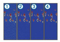
When you adjust the interference setting from off ① through low ②, medium ③, and high ④, noise is gradually removed, but there is little effect on the strong target returns.
