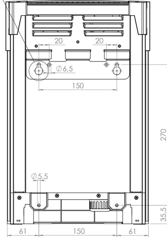
Backside: ChargeMaster III with mounting bracket.
