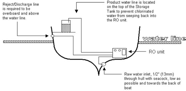
Figure 2.1: Recommended installation **BELOW** waterline.
