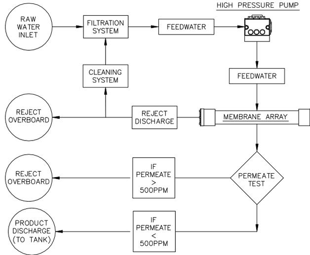
**Figure 3.2: Simplified Schematic of an RO System.**
