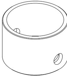
*Fig. 6: Seal Retainer*
