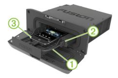
4 Connect the adapter cable to the media player ③, and place it in the device tray. **NOTE:** If you are connecting an Android™ device to the stereo, you should unlock the device before connecting the adapter cable.
